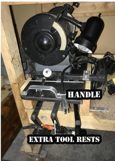
Because I'm in a small shop, space is at a premium my Grinder, Metal Vise, Metal Bender have cleats on the bottom that are secured with my woodworking vise while using them. My Grinder is stored under my worktable. Because of the cleat (tilting the grinder backwards) when I put the grinder away it would catch on the workbench legs. My solution was to raise the Grinder on 2x4's with railings, and add a handle (for more control) to the base. Under the grinder I can store extra tool rests etc.
